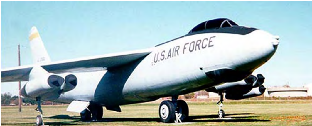
XB-47 46-066 with a modification that installed an "E" nose.
