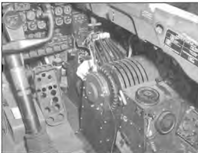
The 7th throttle for the Orenda mounted on the co-pilot's throttle stand in the CL-52.
