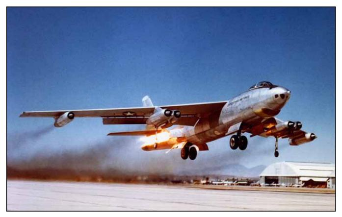
This photo has been often seen but seldom correctly identified. It shows the takeoff of B-47B 49-2644, the testbed for Aerojet's liquid RATO system. Seen here at Edwards AFB in 1954, the system is demonstrated successfully after years of explosions and other problems. Despite the success, the tests were terminated and use of the solid rockets continued until the B-47s were retired.
