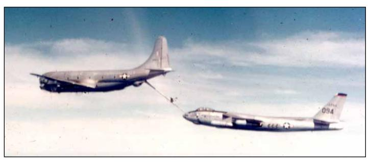
A rare color photo of a TB-47B taking on fuel from a KC-97. Daylight made it easier but it was never easy and at night it Photo: USAF was a whole different story (see article below).
