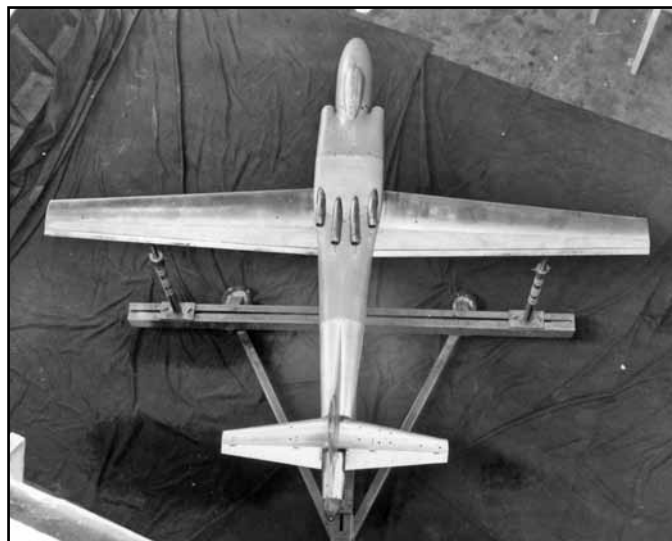
This is an overhead view of Boeing Model 432 showing the fuselage-mounted jet engines with over-the-wing exhaust. This wind tunnel model still has straight wings but that would change after Schairer's letter reached Seattle.
