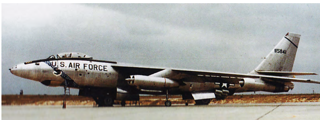
The RB-47E on alert duty (note ATO rack installed)
