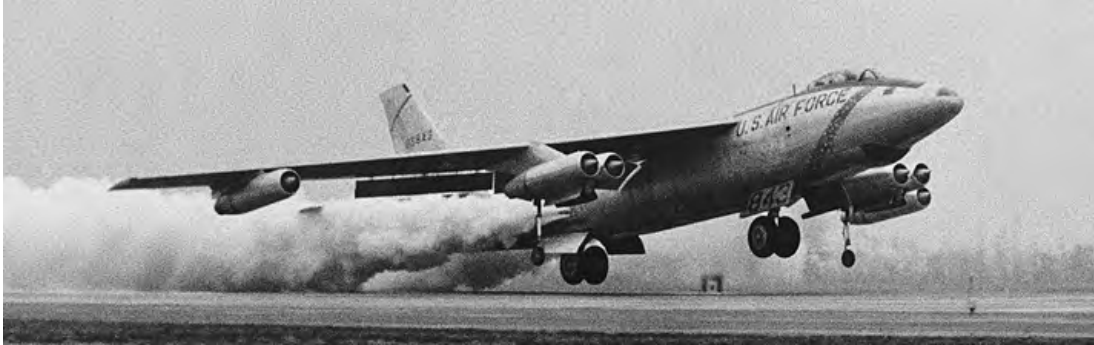
The B-47A using internal RATO
