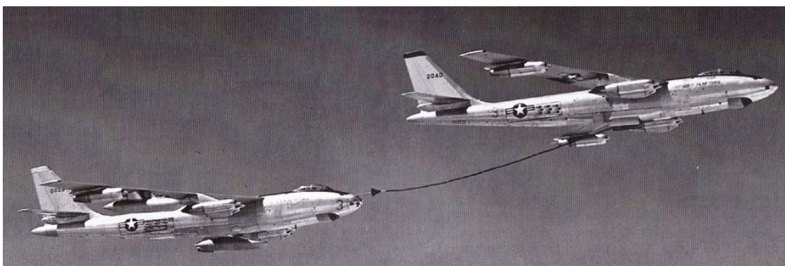
The YB-47F (lower aircraft) refueling with the KB-47G
