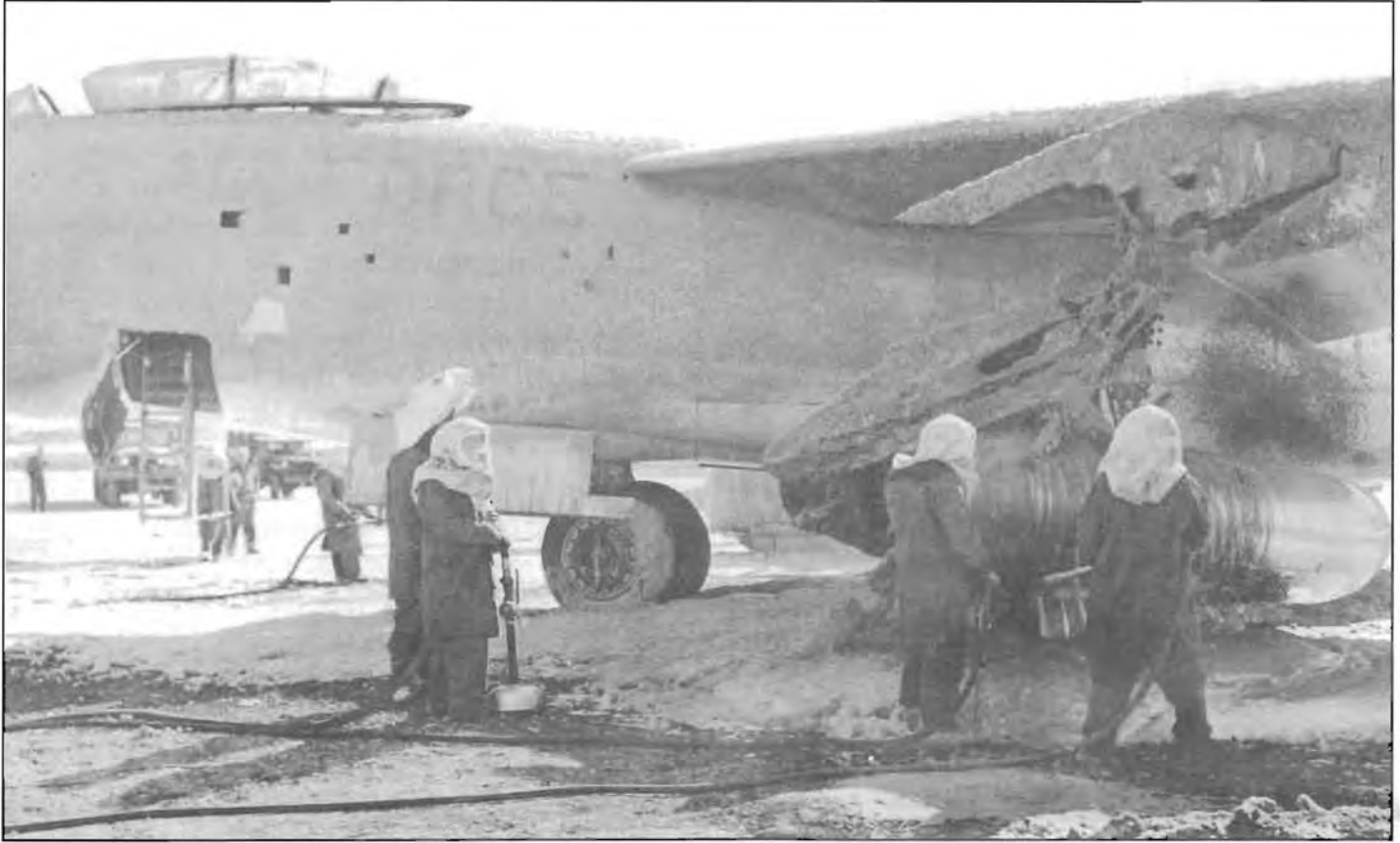
The entry door, with ladder extended, is open after Gordon Daniel and his crewmates abandoned the aircraft, now surrounded by emergency crew. Note the inboard nacelle with its aft end facing forward. Photo: USAF/author
