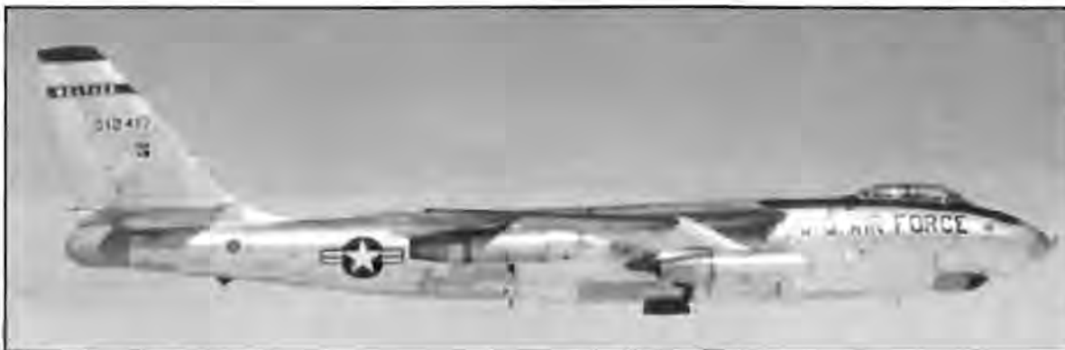
WB-47E, 51-2417. Note scoop mounted on belly. Tail turret was modified to provide space for the nine shot dropsonde dispenser. The inflight refueling capability and bombing equipment were deleted. Photo: via Dick Purdum
