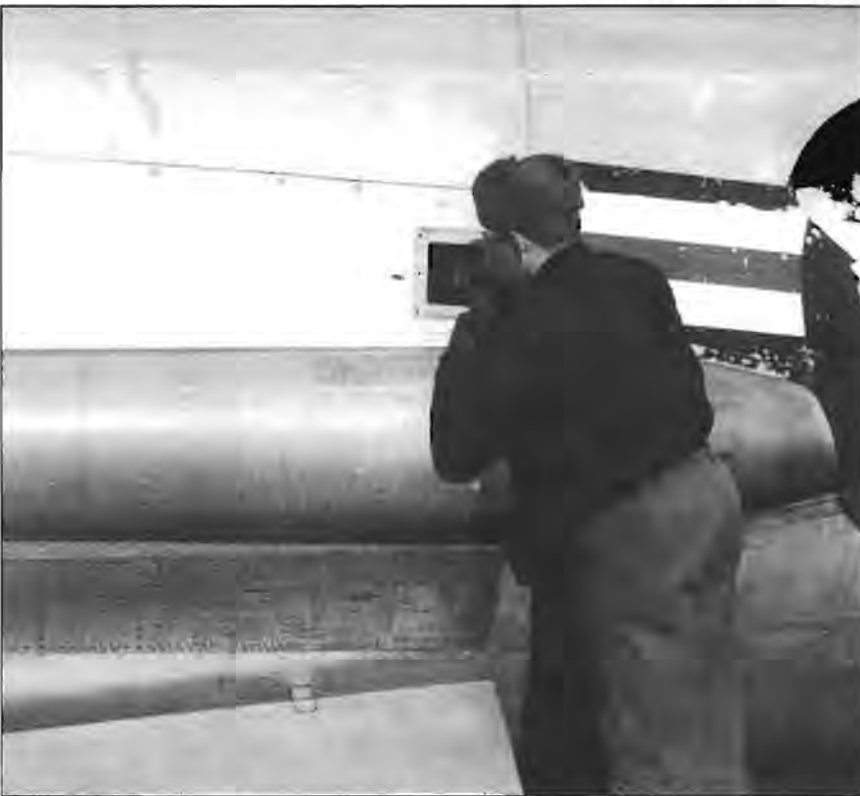
Barney Calligan performing preflight during Operation Snowflurry at Goose Bay AFB. Note the SLAR radome over which he is leaning. The rear landing gear door is just below and the radome actually distorts the national insignia at its aft end. There was an identical radome on the opposite side.
