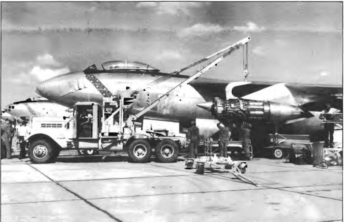
An engine change being performed on an unknown B-47 probably at MacDill AFB. Maintenance wasn't always carried out in beautiful weather such as this. Note this Stratojet has the early sliding canopy and there is no anti-flash paint on the lower fuselage.
