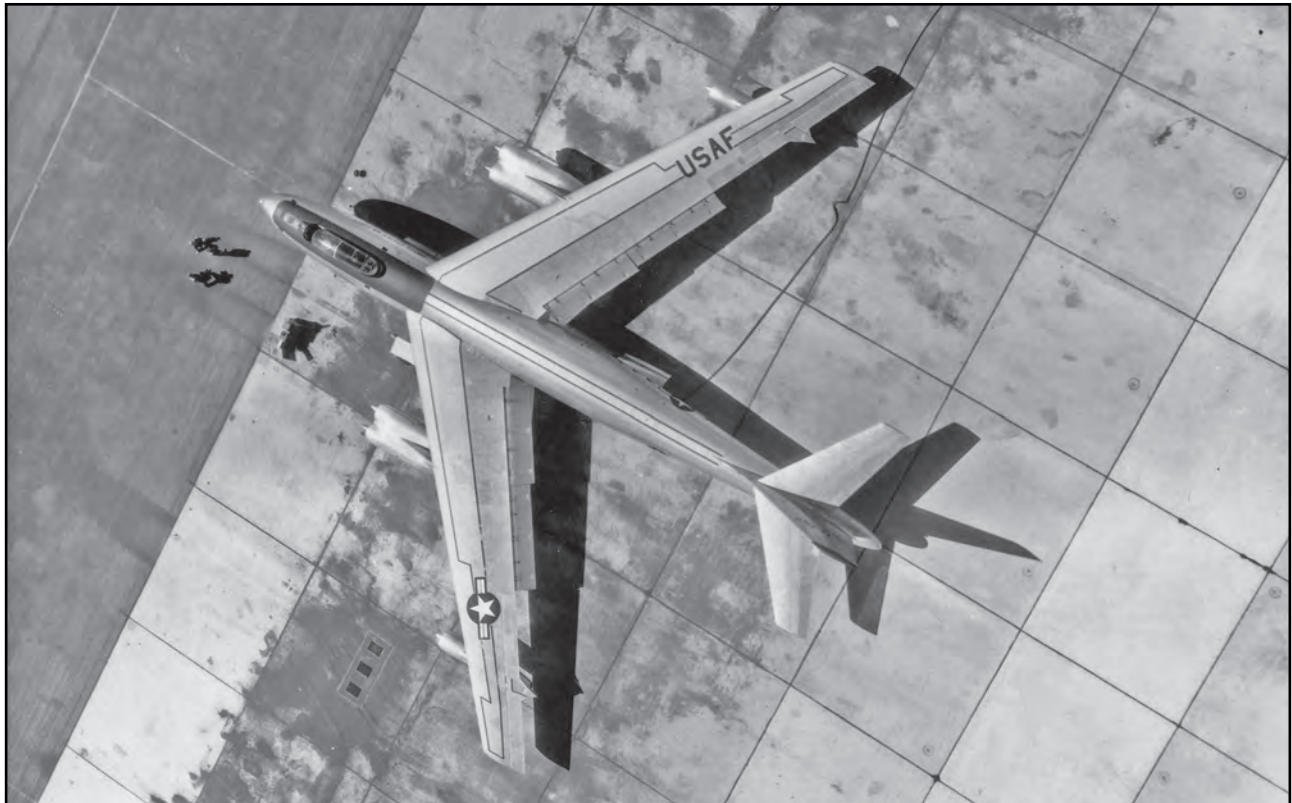
An Unusual view of an early Stratojet. Note there are no wing tanks or tail turret. Photo: USAF
