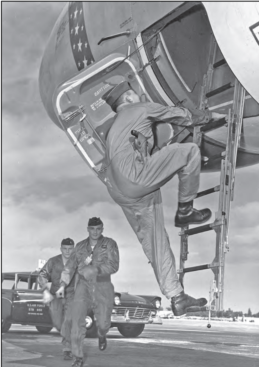
This staged shot of a B-47 crew scrambling to the cockpit shows the features of the door and ladder described by Hooppaw. Note the knob below the lowest rung.
