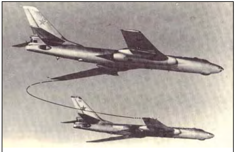
The Soviets adopted an early wingtip-to-wingtip method of aerial refueling that is reminiscent of early procedures in the United States
