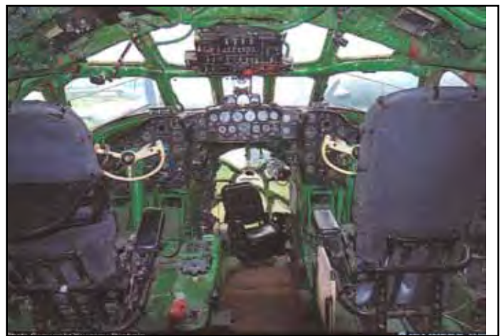
The TU-16 had a cockpit that featured a walk-through entry into the bombardier's compartment. The glazed nose was a feature of many Soviet designs, even some airliners.
