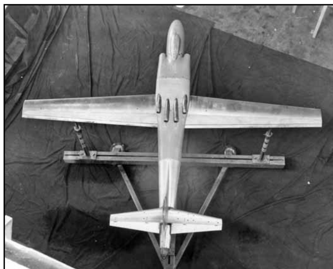
This is an overhead view of Boeing Model 432 showing the fuselage-mounted jet engines with over-the-wing exhaust. This wind tunnel model still has straight wings but that would change after Shairer's letter reached Seattle.
